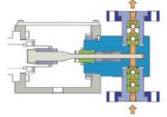
Typical diaphragm pump with double ball valves
