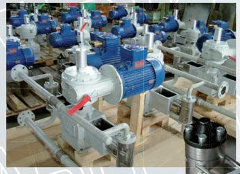
Rod thrust: 1200 kg Stroke length: 60 mm RPM Max: 200
