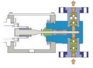
Double diaphragm hydraulic actuated pump "Sandwitch type" with double valve
