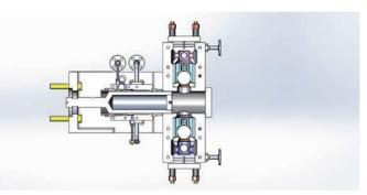
High temperature arrangement with heating jacket and ball valves
